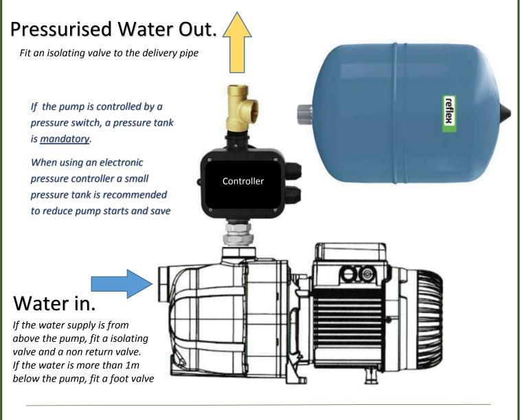
Pressure tank pre-charge when controlled with an Electronic Pressure Controller.
